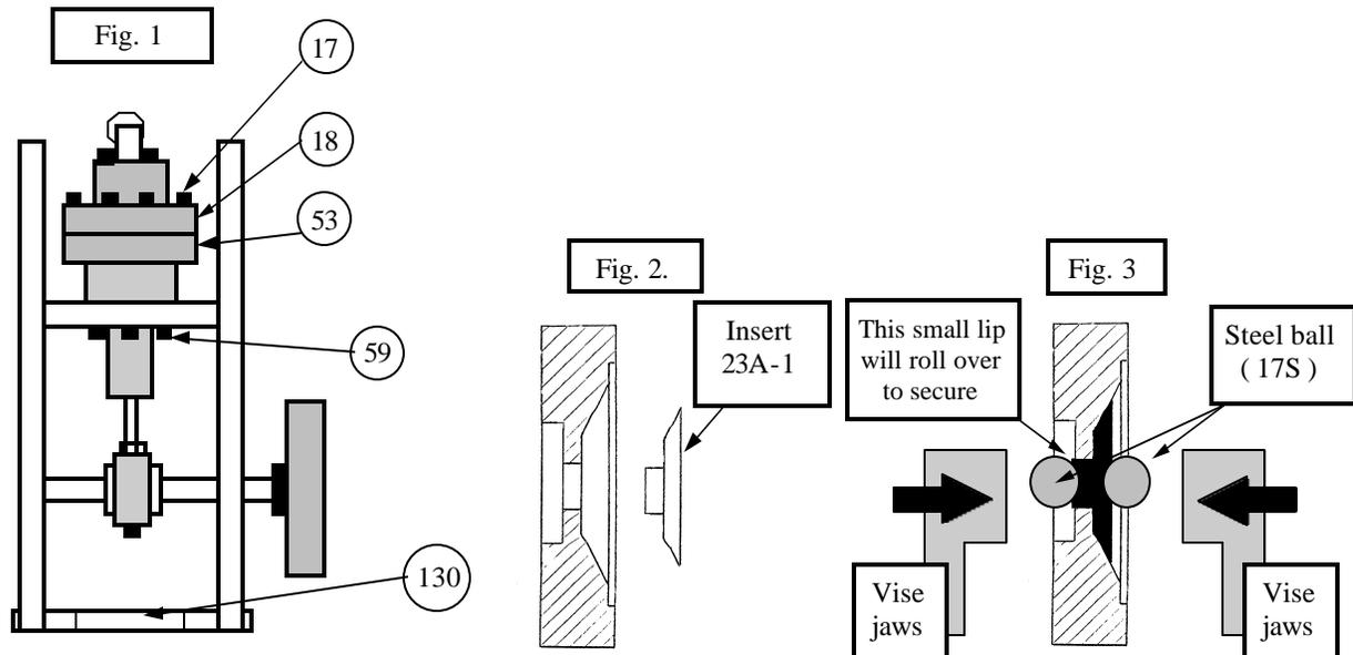
1. Tilt unit up onto its' nose ( resting vertically on handle, ref# 130). See Fig. 1.
